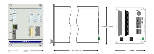
The **AMG5904A966HPG** is a rackmount data receive unit designed to transmit and receive 2 data channels, 6 audio channels, 2 Echelon FTT-10A data channels and 8 bi-directional alarms over one Singlemode optical fibre. It also provides full duplex 100Base-T Ethernet connectivity. The HP suffix in the partno. indicates High Power optical transceivers.
