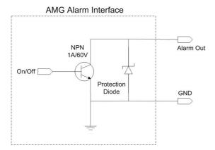
The alarm output circuit is designed for low dc voltage / low current operation and has minimal internal protection. If an alarm output is used to drive an external relay circuit, the external crcuit MUST include a protection (flyback) diode connected across the relay to prevent the high voltage generated from a back EMF causing damage due to the AMG output transistor.
